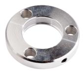
Rigging for all K&M loudspeaker and lighting stands with extension tube diameter of 30-35 mm. Installation using a threaded pin and Allen wrench / hexagon key included in the delivery. The guy wire ring is made from aluminum and has 3 drill holes ø 10 mm to connect the rigging lines.
