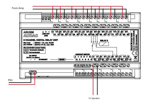
Each of the relays are connected to their own contact within the speakON, and one common ground.
