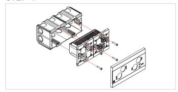
First, plug the twisted pair cable (CATSE or better) into the wall panel. RJ45 port is located on the back of the wall panel. Then, install the wall panel into the single or combined flush mount box by tightening the screws of the wall panel using a screwdriver. Finally, snap and mount the front panel.
