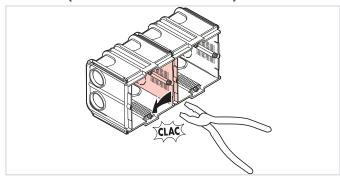
Remove the side walls between the combined flush mount boxes using a plier. This would open enough space for NWP222 to fit in.
