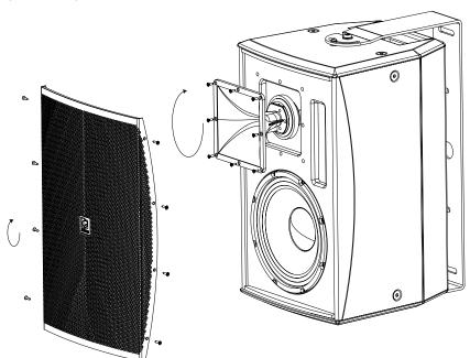
To rotate the VEXO1xxA's horn, the grille must be removed first. To do this, the eight screws on the sides must be unscrewed.
