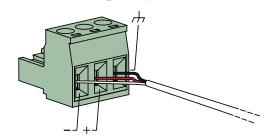
For unbalanced signal input connections
