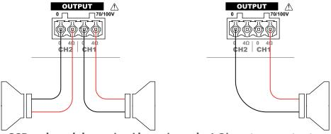
SCP series minimum load impedance in 4 Ohm stereo output mode
