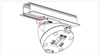
When inserted in the rail, slide the lock on the side to counter-clockwise and lock it.
