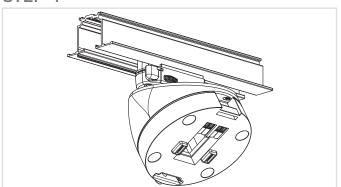
The light track adapter is now locked in place and ready for getting the ATEO4M speaker assembled. Mount the ATEO4M speaker to the combined CleverMount+™ and RMA45M. ATEO4M has two connection latches on it and those connection latches should be placed to attachment points on CleverMount+™ mounting system.
