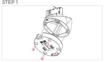
The first step is mounting the supplied wall mount to the light track adapter mount. The wall mount has to be fixed by four screws in a quadrangular shape. Distance between mounting holes are shown ATEOXM User Manual.
