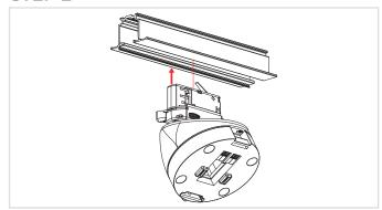
The the combined mounting system can be inserted through the light track rail directly as can be seen in the visual.
