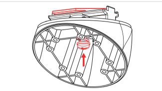
Press the bolt and spring in the center position of the adapter, making the inner metal part of the adapter moving out of the surrounding part.
