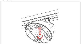
When inserted, release the bolt and tighten it for a more stable fixation. The light track adapter is now locked in place and ready for getting the ATEO4 speaker assembled. Mount the wall plate of the ATEO4 speaker to the RMA40 through inserting and tightening the 4 screws to the provided holes.
