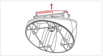
The inner metal part moves out of the surrounding part and can be inserted through the light track rail by aligning it with with the slot opening (rotating about 30° counterclockwise).
