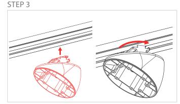
When aligned, slide the adapter in the rail and lock it in place through pushing it inside and giving it a 30° clockwise rotation. STEP 2
