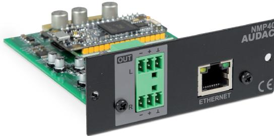
The NMP40 is a SourceCon™ compatible module featuring an (internal) board–edge connector which carries all signals for getting it connected to any supporting main unit.
