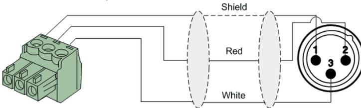
For unbalanced line output connections:
