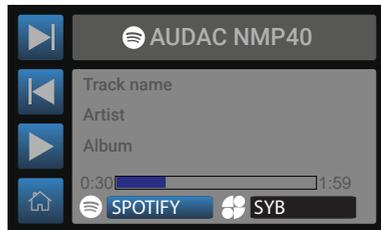
The left section of the screen indicates 4 quick buttons which can be controlled through the tactile buttons on the left screen side. Switching between the streaming services is done through rotation of the rotary dial and pressing it when the desired service is highlighted.
