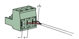
For unbalanced line input connections.
