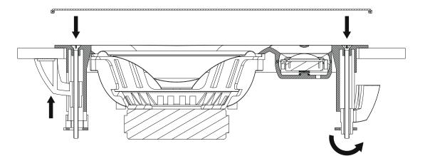
6) After the screws are tightened and the speaker is level with the surface, the front grill can be assembled to the loudspeaker.
