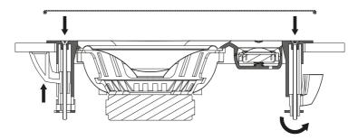
6) After the screws are tightened and the speaker is level with the surface, the front grill can be assembled to the loudspeaker.
