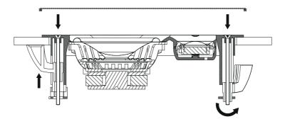
6) After the screws are tightened and the speaker is level with the surface, the front grill can be assembled to the loudspeaker.
