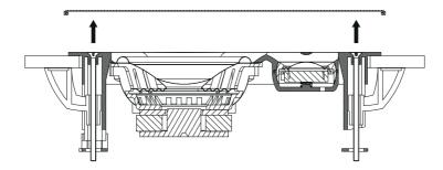
4) Connect the loudspeaker connection cable to the gold plated spring clamp connectors. Press the button of the corresponding terminal down and insert the connection cable. After releasing the button, the cable is connected to the loudspeaker. The Red terminal indicates positive (+) pole and the Black terminal indicates the negative (–) pole.
