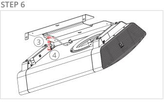
Mount the loose end of the safety wire to the safety bracket and make all electrical connections
