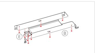
Attach the ceiling plate and the safety cable bracket in the desired location using the appropriate screws for your mounting surface.
