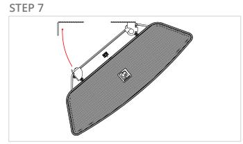
Rotate the other end of the NOBA8(A) up until the holes of the ceiling bracket line up with the holes on the NOBA8(A) bracket.
