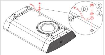
Attach the safety cable to the NOBA8(A) chassis
