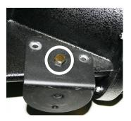
Mark the two other holes, remove the brace and drill the marked holes.
