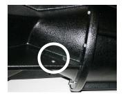
Place the brace over the hole in the side of the speaker. The hole in the speaker should correspond with the middle hole in the brace.
