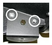
Place the brace back and fix it with three bolts.
