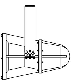
• Wall mount (minimum of 3 mounting points should be used, including the 2 most outward holes)
