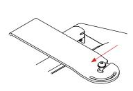
Insert the large (M10) bolts through the rubber washer and into the center threaded holes (top and bottom). This washer comes between the speaker and the bracket.
