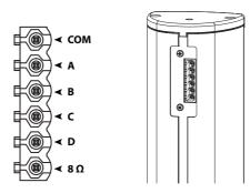
When using in constant voltage 70/100V systems, the power taps can be adjusted in 4 steps of impedance through connecting the appropriate terminals of the 6-pin terminal block connector. Each position corresponds with a specific impedance / power setting indicated on a label attached to the speaker, and in the table below.
