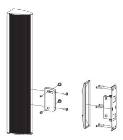
It consists of two different parts, whereof the first part should be installed to the rear side of the loudspeaker. It can be assembled on different heights on the rear of the speaker, depending on the mounting possibilities and required installation height. It is fixated to the loudspeaker cabinet by inserting the 2 supplied mounting screws into the pre-drilled and threaded holes at the back of the speaker cabinet.
