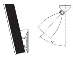
Once installed, the speaker can be can be panned and tilted, focussing the loudspeaker into the desired listening direction. This is useful when the installation height on the wall is limited or the speaker is mounted from the side. The maximum downward tilt is  $13^{\circ}$  and the maximum pan in both directions is  $42^{\circ}$ .
