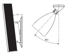
Once installed, the speaker can be can be panned and tilted, focussing the loudspeaker into the desired listening direction. This is useful when the installation height on the wall is limited or the speaker is mounted from the side. Depending on the selected speaker part, the downward tilting angle can be adjusted within a range of 0° and 6.5°, or within a range of 6.5° and 13°. The maximum pan in both directions is 42°.
