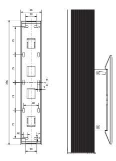
Once both speaker part and wall part are safely attached to their positions, the protective finishing cover can be assembled over the wall plate by clicking it. Afterwards the speaker can be assembled to the wall bracket by bringing both parts together and tightening them through the button head bolt and nuts together through an hex drive key. The upper one can be used for adjusting the tilt–angle of the speaker.
