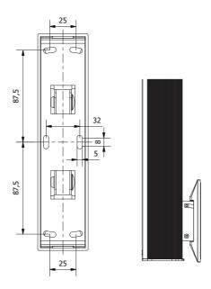
Once both speaker part and wall part are safely attached to their positions, the protective finishing cover can be assembled over the wall plate by clicking it. Afterwards the speaker can be assembled to the wall bracket by bringing both parts together and tightening them through the button head bolt and nuts together through an hex drive key. The upper one can be used for adjusting the tilt—angle of the speaker.
