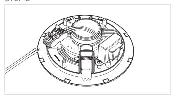
Connect the wires coming from the amplifier to the SnapConnect™ on the rear of the loudspeaker.
