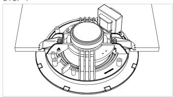
Insert the speaker through the provided ceiling cutout, make sure the spring loaded mounting arms are behind the clamping surface and release them. The ceiling is clamped between the mounting arms and the speaker baffle and is installed correctly.
