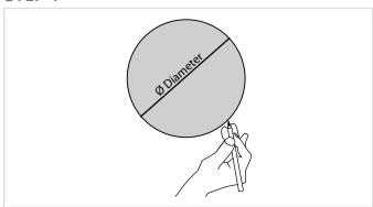
Cut a hole on the desired mounting location in the ceiling. Make sure the dimension is matching the cut-out measurement for the installing loudspeaker
