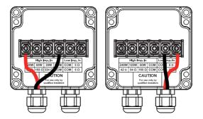
Above image indicates an example for both a 100V (left side) and low impedance (right side) connection example.
