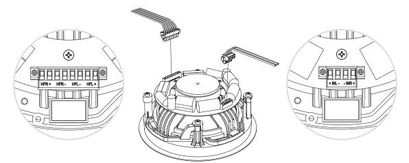
4) Make sure the mounting clamps are fully bended inwards, allowing the speaker to fit through the cut out. Insert the speaker into the cut out and tighten the mounting screws. A quarter turn is enough to flip out the mounting clamps, locking the speaker in place.
