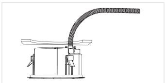
Make sure the spacing between the mounting surface and the clamp is bigger than the thickness of your ceiling plate. Insert the speaker until the clamps snap in place
