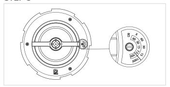
Using a flat head screwdriver, the power tap selection can be made in various tappings for 70/100V or low impedance (8 $\Omega$ ) use. Use the correct scale (70V or 100V) for the power tap selection according to the line voltage being used in your system.
