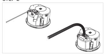
Open the swivel lid and connect the cables to the terminal block connector by inserting the cable in the corresponding hole and tightening the screw. The remaining two terminals can be used to link through to other speakers.
