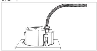
Fix the speaker in the provided opening by tightening the screws of the mounting clamps using a screw driver. An optional tile bridge must be installed when mounting the speaker in ceiling tiles.
