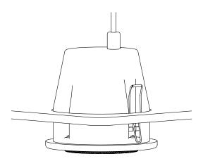
3) When the speaker is mounted, push both springs downwards to lock the speaker in in place. Once the springs are pushed down, the speaker will place itself properly in line with the panel. In this image the AWPO6 speaker is locked tightly and ready for use.
