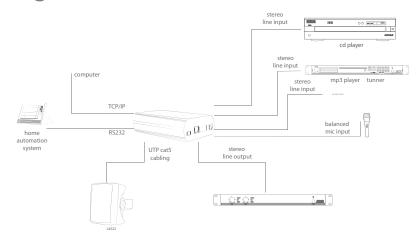
When connecting the LX523 speaker system to an RM523 Web based input control unit, both devices use RJ45 in- and output connectors. In this case, just a regular CAT5 cable (or better) should be used, on both sides terminated with an RJ45 plug. The connection way of this cable should be 'Straight', according to the colour standard described before in this user manual.
