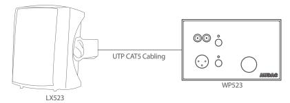
In the most common applications the LX523 active speaker system will be used in combination with the WP523 wall panel. This wall panel contains an unbalanced line input (RCA) and balanced microphone input (with phantom power). Both input channels have local mixing which can be controlled through the push-lock potentiometers, and the master volume can be controlled by means of the big dial.
