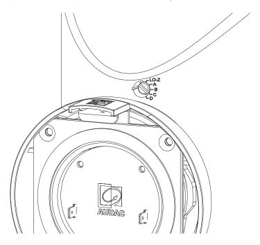
When using in constant voltage 70V/100V systems, the power taps can be adjusted in 4 steps of impedance through selection of the correct connection terminals indicated with A, B, C & D. Each position corresponds with a specific impedance / power setting indicated on a label on the wall plate and in the table below.
