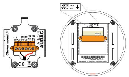
In most cases, the speaker cable will be provided through the wall, making the cable completely invisible from outer side. In some cases, the cable should be fed from outer side. For this purpose, a spot (marked in RED) with thinner material is provided at the bottom side, which can be removed using a plier for feeding the cable into the circular bracket.
