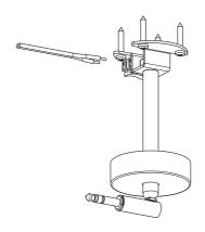
Once connected, the ceiling cover can be slided and clicked in place, nicely covering the screws and connections. Mind the direction of the fixation clips at the inner side of the cover, to make sure they nicely get into place when pressed onto the bracket.
