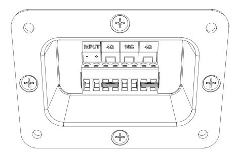
16 Ohms: Single connection bridge between 16 Ohm terminals.
