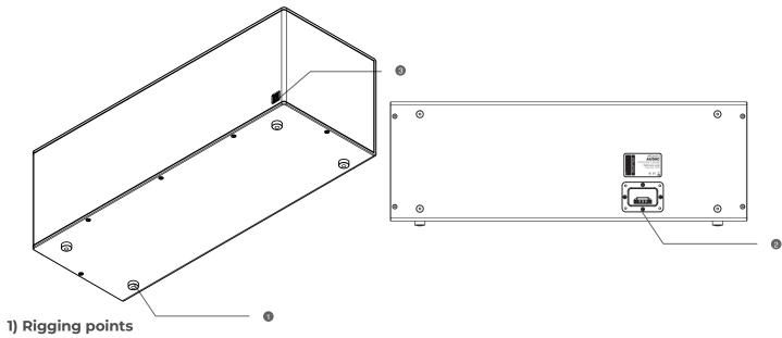
Rigging points are available on ARCHI series for optional mounting brackets. These brackets allow flexible and secure mounting on walls and ceilings to achieve an architectural discreet pleasing installation.
