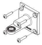
Once this part is correctly mounted to the desired location on the wall or ceiling, the cabinet can be assembled to the bracket. This is done through inserting the supplied bolt (M6) through the hole in the bracket (speaker part) and tighten it into the wall or ceiling part.
