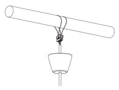
The ALTI speakers are delivered with a ceiling cover, which covers the fixation points (snap hooks or Gripple® connectors) on the ceiling side, in case a clean finishing is required. Slide this ceiling cover over the connection cable first, before any connections or fixations are made.
