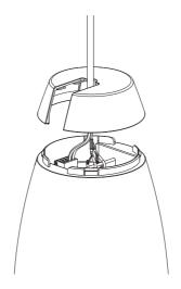
Once assembled, the sliding tab can be inserted to the cover and can be slide into position, offering a nice and clean outlook of the cabinet.
