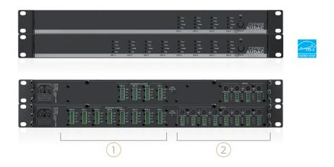
The CEP series are professional 70/100V multichannel energy-efficient amplifiers. The one unit height device comes into two models. The CEP408 offers four channels and has an output power of 80 Watt. Both low impedance as 70/100V, deliver high-quality amplification distributed over multiple zones in various applications.
