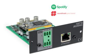
The NMP40 SourceCon™ Network audio player module enables the possibility to stream audio files from a personal computer or mobile device directly to a professional audio system while maintaining the best available sound quality.
