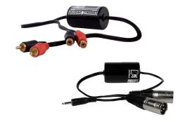
The TR2000 series are basic stereo groundloop isolators, designed as problem solvers to electrically isolate audio devices from each other. Hum in audio systems is usually caused by groundloops in the system. The most common and simple method to solve these problems is an audio isolation transformer such as the TR2000 series.
