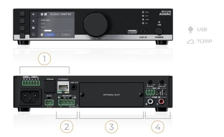
This all-in-one solution is designed as a two-channel amplifier using class D amplifier technology. It can be used for powering low impedance stereo systems with a maximum power of 2 x 80 Watt, while bridging to a constant voltage (100V and 70V) is possible with a maximum output power of 160 Watt. A switch-mode power supply allows a wide variation of mains voltages for global compatibility.
