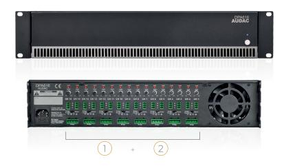
Its size makes this dual rack space amplifier ideal for multi-zone audio distribution systems with up to 8 stereo or 16 mono zones. Its use of Class-D technology ensures excellent efficiency as well as outstanding sound quality. For added reliability, an advanced circuitry protects them against DC malfunctioning, short circuiting, overheating and overloading.
