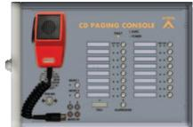
The unit offers "Hold" and "Busy" LED signals in addition to the zone LED's, and these allow the easy identification of selection / Busy signals for the user. In addition, to comply with EN 54-16, separate POWER, FAULT and EVAC indicators are provided.
