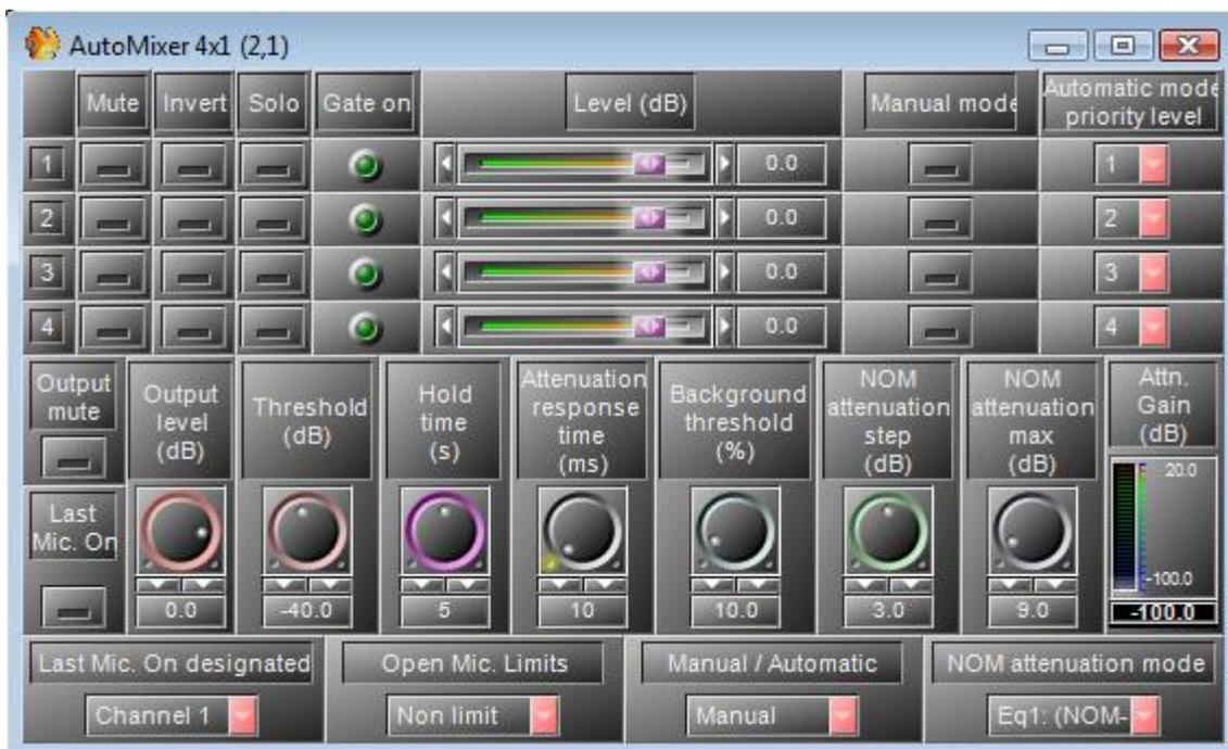
The auto mixer adjusts the signal output level on the output node depending on the number of activated input channels. This function can be useful in conference applications or houses of workshop, where usually unattended mixing has to be executed.
