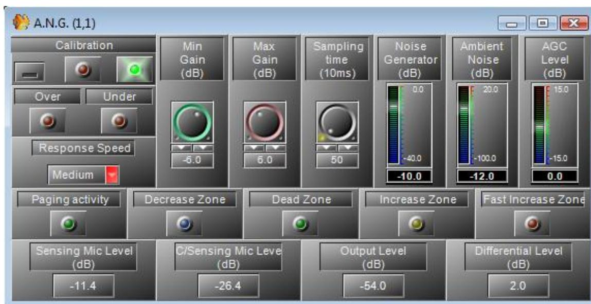
Now the A.N.G will automatically adjust the level on the (P.M) signal depending on the ambient noise detected on the sensing microphone.
