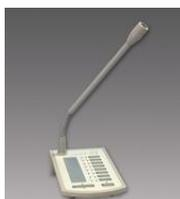
Same features as the PPM and a small memory (2min audio) in the PPM-SP allow storing the message if the PPM-SP cannot route the message to the desired zone. When the zone becomes available the message will be played.
