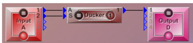
**Threshold:** set at -18dB, because less would active the attenuation when the speaker is not talking if the microphone catch some unexpected noise.
