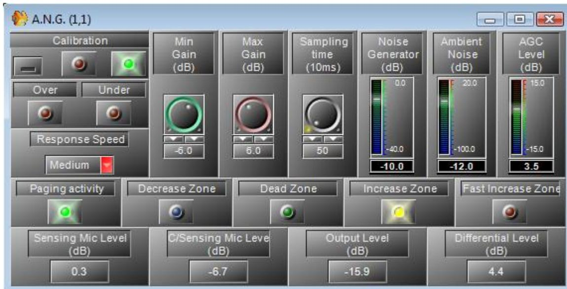
In our example, the noise is now louder than during the calibration. The differential level is around 4.4dB.
