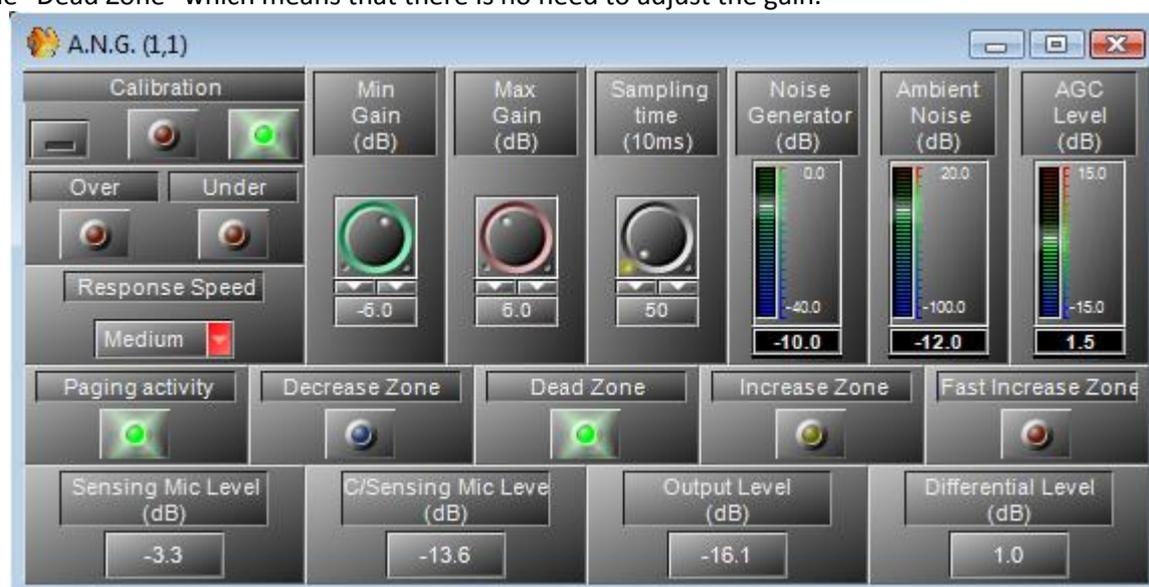
As the noise level is near than during the calibration, the differential level is almost null.
