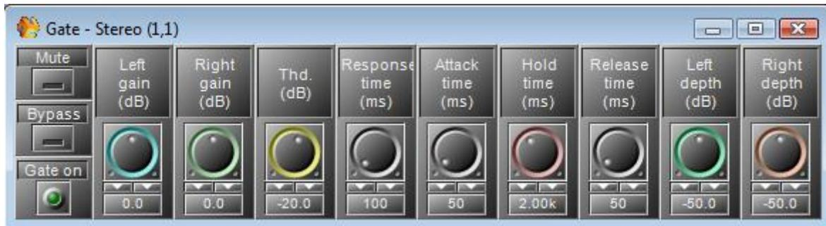
When one of the inputs goes above the threshold, the gate becomes active and the both left and right input signals are routed to the output.
